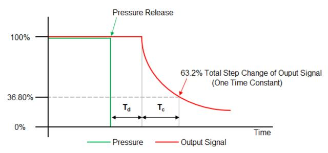
Mechanical response time (MRT) is the time it takes for the process pressure change to be conveyed mechanically from the diaphragm to the sensor. MRT can be affected by any number of mechanical factors - spring rate of the diaphragm (which is different for different materials), the type of fill fluid used to convey pressure to the sensor, or the amount of fill fluid.
